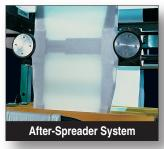
For uniform fabric width control and enhanced drying efficiency
