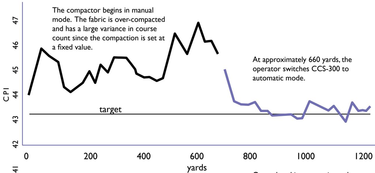
Once placed in automatic mode, the compaction was immediately reduced. CCS-300 adjusted the course count to the desired set point and maintained it through the entire process.
