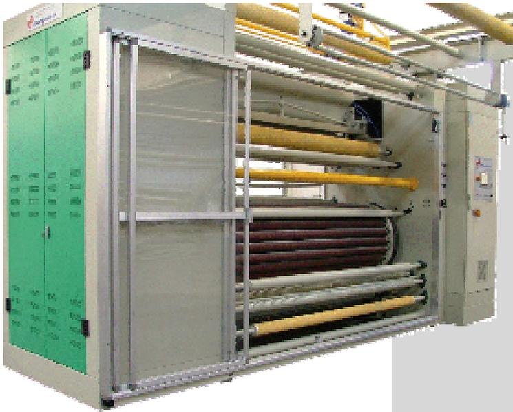
The combing-shearing machine RS5000 introduces a new concept in the processing of raised fabrics that have to be sheared obtaining the anti-pilling effect. Thanks to the combination of a powerful combing system and a shearing unit, it is possible to obtain the highest quality results in the shearing of pile.
